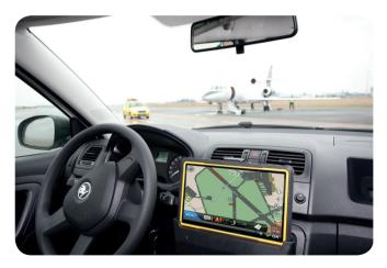
Navigation, information and communication unit of the TE-VOGS system. The unit consists of a tablet with client software located in the docking station in the driver's cabin and of the roof extension with a communication facilities for the wireless network and GNSS receiver.
